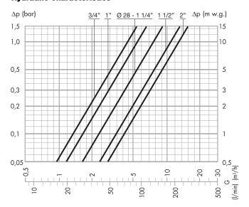
Recommended FLOW RATES to ensure stable operation and accuracy of  $\pm$  2°C (balanced Hot/Cold pressures)
